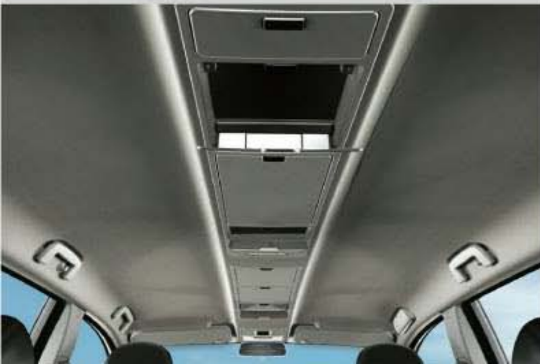
Roof Utility bins
